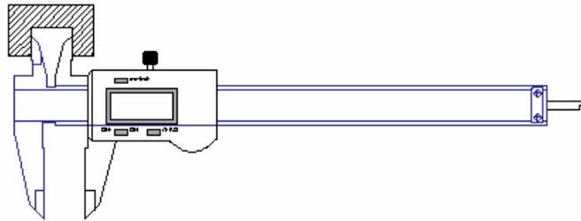
It's a little harder to keep things lined up correctly when you are taking an inside measurement. Be sure that the calipers are not cocked, or you will not get an accurate measurement.
