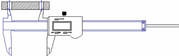
Be sure to use the same (inside) jaws for both measurements. And remember that this works only if the holes are the same size.
