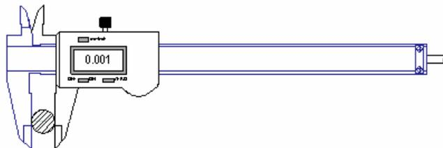
The caliper shows you how much material you need to remove, from either the shaft or the hole, to make them fit.
